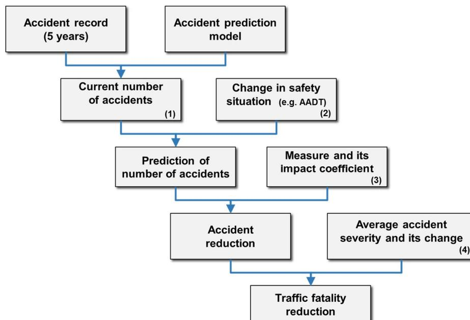
Fig. 1. Evaluation of traffic safety effects of road improvements, using TARVA (Peltola et al., 2013).
